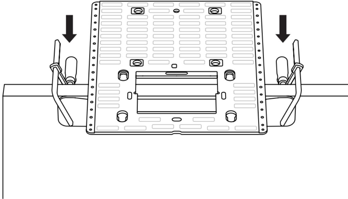
**The markings on the top face of the Edge Mortising Adapter align with Plate's reference points.**
