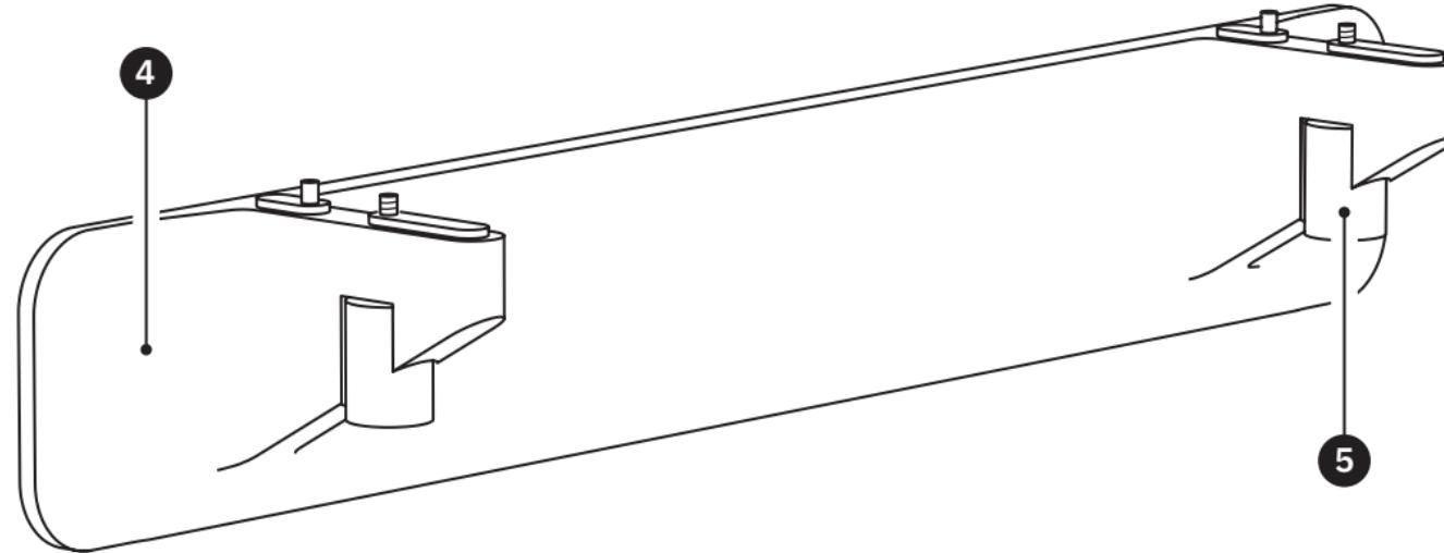
**Place Plate on a flat surface, reverse side up. Align the locating pins and mounting screws with the corresponding holes on Plate's side rails and tighten the screws.**
