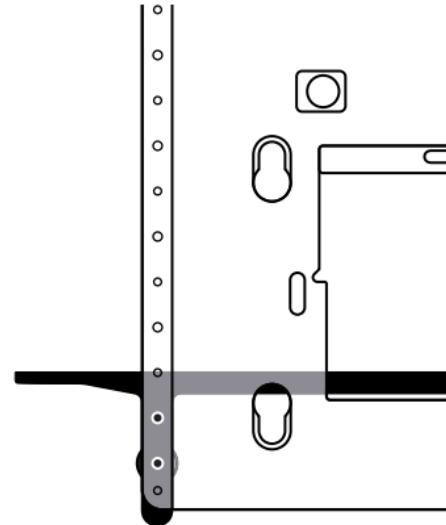
**Secure Plate to your workpiece using clamps. place your clamps at a slight angle so that they do not impede you while cutting. *Clamps not included.***
